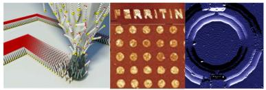
Left: Scheme representing the DPN deposition process using a functionalized AFM probe. Middle: Nanoarrays of protein ferritin and word fabricated on gold with DPN. Right: Circular pattern of nanomagnets integrated on a µSQUID device with DPN.
